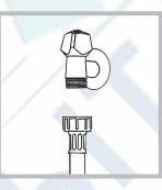
1. Connect the inlet hose by screwing it to a cold water tap using a 3/4 gas threaded connection *(see figure)*. Before performing the connection, allow the water to run freely until it is perfectly clear.
