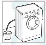
electrical socket. 2. make sure the water level inside the machine is lower than the door opening; if it is not, remove excess water using the drain hose,
